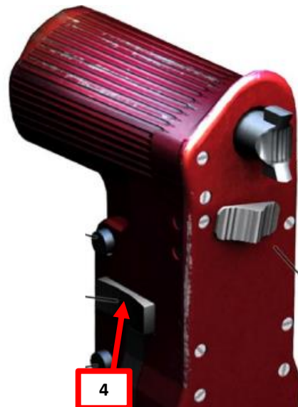
Radio Selection Switch (selects either COM1 or COM2 radio) • UHF Red COM2 Radio Control • V/UHF Green COM1 Radio Control
