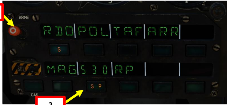
Missile Launched, Lost Lock PSIC Super 530 + Forced Illumination Mode
