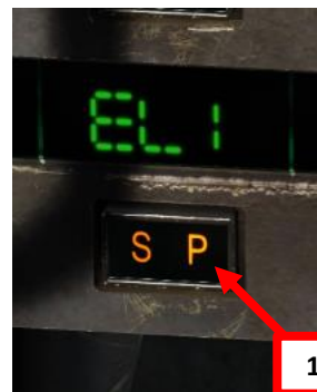
10a Weapons System CMD Switch FWD
