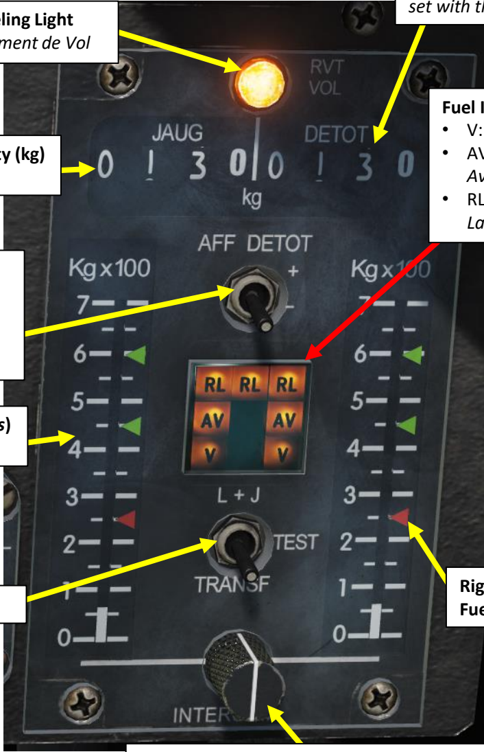
Internal Fuel Transfer Control (Not Functional) • Fuel cross-feed, used to keep fuel level balanced for different fuel tanks
