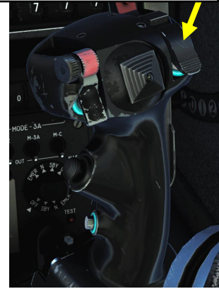
MAGIC Search / Vertical Fix Button (Nav Update / Magic Unlock) (can be used to switch Magic II Search Mode)
