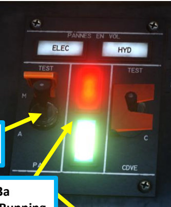
33a PA Test Switch – Marche (ON)
