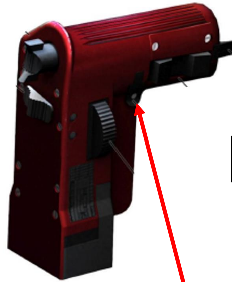
25 Magic Slave / Air-to-Ground Designate Button
