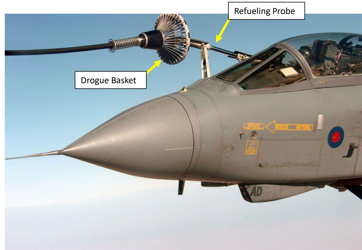
Tornado GR4 being refueling by a Probe-and-Drogue system
