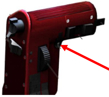
Magic Slave / Air-to-Ground Designate Button 11b
