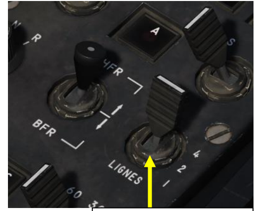
Radar Number of Lignes (bars) selector • (4/2/1)
